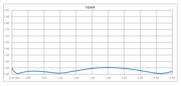
Click the following link (or enter part number in "SEARCH" on website) to obtain additional part information including price, inventory and certifications: 7/16 F/F Bulkhead Coaxial RF Surge Protector, 698MHz - 2.7GHz, 1000W, IP67, 60 V Max., 25mJ, 20kA, Filter, Low PIM -155 dBc TSXDC-DFF
