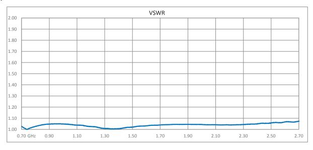
Click the following link (or enter part number in "SEARCH" on website) to obtain additional part information including price, inventory and certifications: Type N F/M Bulkhead Coaxial RF Surge Protector, 698MHz - 2.7GHz, DC Block, 500W, IP67, .005uJ, 40kA, Filter, Low PIM -155 dBc, Hole Mount TSX-NFM-P
