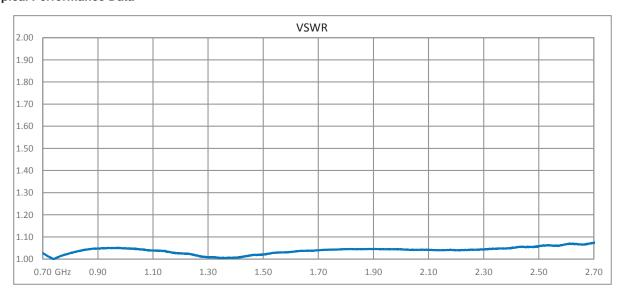
Click the following link (or enter part number in "SEARCH" on website) to obtain additional part information including price, inventory and certifications: Type N F/M Bulkhead Coaxial RF Surge Protector, 698MHz - 2.7GHz, DC Block, 500W, IP67, .005uJ, 40kA, Filter TSX-NFM-BF
