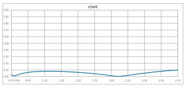
Click the following link (or enter part number in "SEARCH" on website) to obtain additional part information including price, inventory and certifications: 7/16 F/M Bulkhead Coaxial RF Surge Protector, 698MHz - 2.7GHz, DC Block, 500W, IP67, .005uJ, 40kA, Filter, Low PIM -155 dBc TSX-DFM
