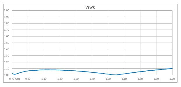
Click the following link (or enter part number in "SEARCH" on website) to obtain additional part information including price, inventory and certifications: 7/16 F/F Bulkhead Coaxial RF Surge Protector, 698MHz - 2.7GHz, DC Block, 500W, IP67, .005uJ, 40kA, Filter, Low PIM -155 dBc TSX-DFF
