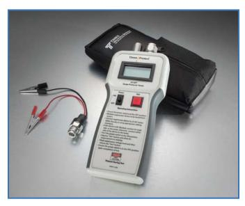
The Times Protect LP-SPT Surge Protection Tester is designed to test all coaxial cable RF Lightning Protection products offered by Times Microwave. Other LP products based on transient protection devices such as GDT, MOVS, TVS and SIDACs and mechanical filter designs can be tested. Moreover the LP-SPT is suitable for testing discrete transient devices as well.
