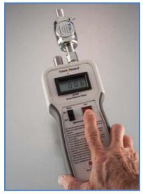
A **dc blocked protector** must be tested with the **surge side connector** attached to the LP-SPT. The protector can remain physically mounted with the equipment jumper attached. *Turn off equipment!*
