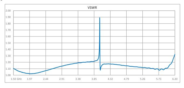
Click the following link (or enter part number in "SEARCH" on website) to obtain additional part information including price, inventory and certifications: Type N F/M Bulkhead Coaxial RF Surge Protector, 1.8GHz - 6GHz, DC Block, 10W, IP67, .5uJ, 18kA, Filter LSXL-ME
