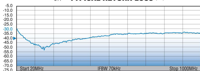
S11 TYPICAL RETURN LOSS (dB)
