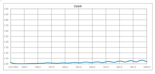
Click the following link (or enter part number in "SEARCH" on website) to obtain additional part information including price, inventory and certifications: Type N F/M Bulkhead Coaxial RF Surge Protector, 10MHz - 1GHz, DC Block, 1.5kW, 3.5mJ, 20kA, Blocking Cap, Hole Mount IS-B50LN-C0-ME
