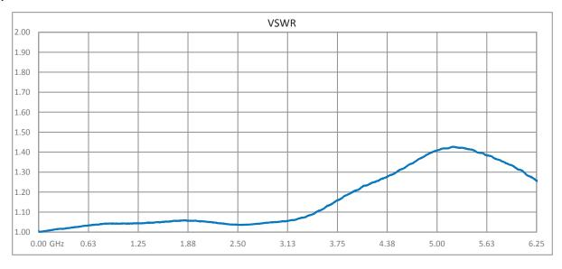
Click the following link (or enter part number in "SEARCH" on website) to obtain additional part information including price, inventory and certifications: Type N F/M Bulkhead Coaxial RF Surge Protector, DC - 6GHz, 1000W, IP67, 6 V Max., 2.5mJ, 20kA, Gas Discharge Tube GTH-NFM-AL
