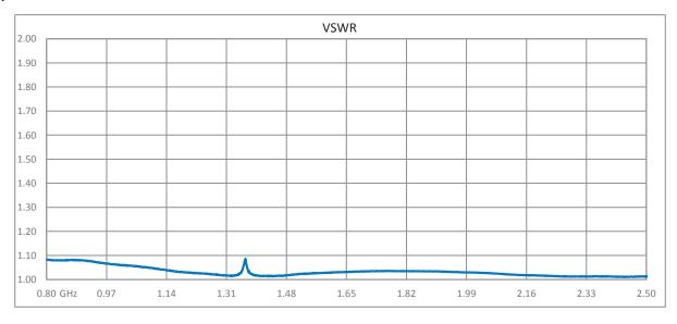
Click the following link (or enter part number in "SEARCH" on website) to obtain additional part information including price, inventory and certifications: Type N F/F Bulkhead Coaxial RF Surge Protector, 800MHz - 2.5GHz, 300W, IP67, 6 V Max., 16uJ, 20kA, Hybrid DGXZ+06NFNF-F
