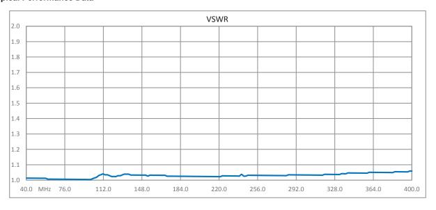
Click the following link (or enter part number in "SEARCH" on website) to obtain additional part information including price, inventory and certifications: Type N F/F Coaxial RF Surge Protector, 40MHz - 400MHz, 100W, IP67, -6 V Max., 2.5mJ, 20kA, Hybrid, Bracket Down, Hole Mount BGXZ-60NFNF-ALT
