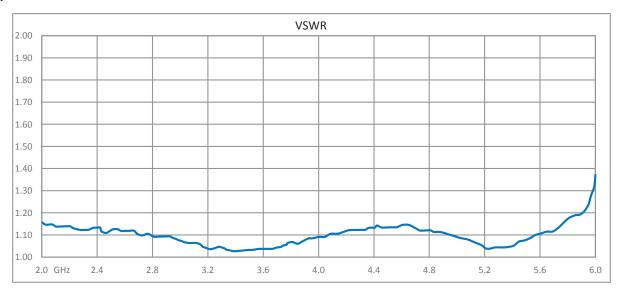
Click the following link (or enter part number in "SEARCH" on website) to obtain additional part information including price, inventory and certifications: Type N M/F Bulkhead Coaxial RF Surge Protector, 2GHz - 6GHz, DC Block, 10W, IP67, .5uJ, 10kA, Filter AL-LSXM-MA
