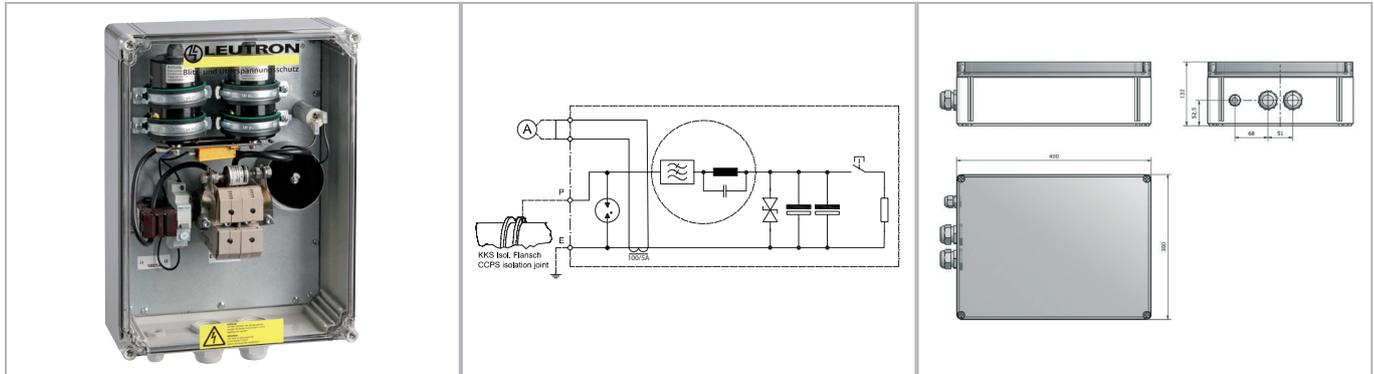
With an active cathodic corrosion protection the installation is permanently protected against the electrochemical process of corrosion. For that matter a grid supplied rectifier is inserted between the installation (e.g. a pipeline) and an anode that serves as earth electrode. By connecting two or three PLPro units in parallel the overall current can be elevated up to 80 respectively 120 A.
