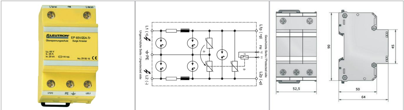
Two-pole USP for operating currents up to 20 A and a nominal impulse discharge current of 20 kA (8/20 $\mu$ s) for sensitive electronic devices.
